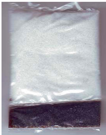
Fig. 1. Laundry detergent sachet. Top half contains 12.5 g of oxalic acid and the bottom half contains 1.2 g of \text{KMnO}_4 .
